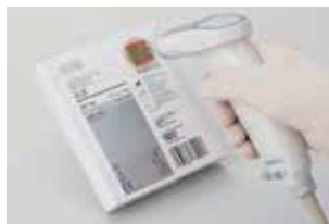
Calibration by scanning a QR code
