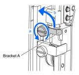
4 Loosen the screw of the bracket B by hand (a) and then remove the bracket B (b).
