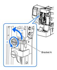
**3** Hold the tube at the top of the piercing nozzle, and pull upwards and remove the tube.
