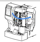
Occording to the bracket A by hand (a) and then turn the bracket A in the direction of the arrow (b).
