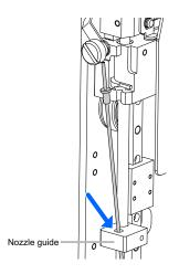
Tit the protrusion at the top of the piercing nozzle into the recess in the nozzle holder.
