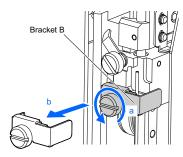
**6** While holding the top of the piercing nozzle, pull the nozzle slightly forward.
