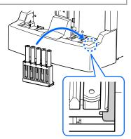
Up to 2 normal racks can be loaded onto the loading side.
